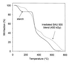
Figure 3. Plots representing the weight loss of native starch and irradiated SAU50 blend submitted to thermogravimetric analysis in air at a heating rate of 10°C.min<sup>-1</sup>.
