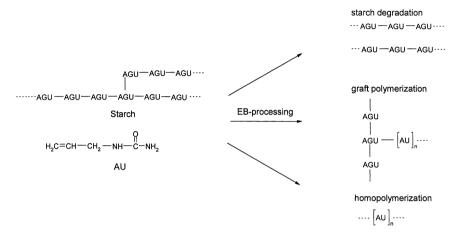
Scheme 1 - Simplified representation of the reactions induced by the EB-treatment in starch - allyllurea (AU) blends [AGU for anhydroglucose unit].
