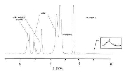
Figure 5. <sup>1</sup>H nmr spectrum (300 MHz, d-DMSO) of the water - methanol insoluble fraction of an irradiated SAU50 treated with a 400 kGy EB dose.
