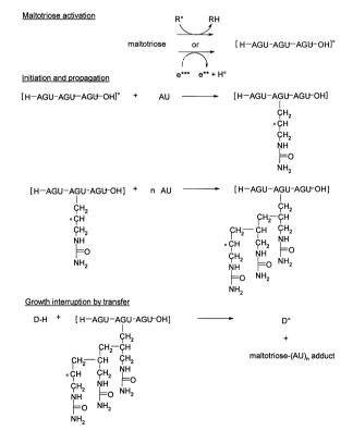
Scheme 3. Proposed mechanism for the graft polymerization of AU onto maltotriose under EB irradiation.
