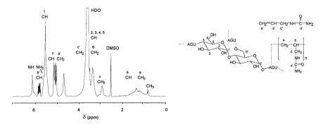
Figure 4. <sup>1</sup>H nmr spectrum (300 MHz, d-DMSO) of an SAU50 blend after EB processing with a 750 kGy dose.
