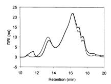
Figure 7. SEC traces of a mixture of maltodextrine (100 wt-parts) and AU (50 wt-parts) mixture before (---) and after (—) 400 kGy irradiation in the solid state.
