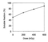
Figure 6. Variations of the soluble fraction of material in water, after irradiation of SAU50 blends.
