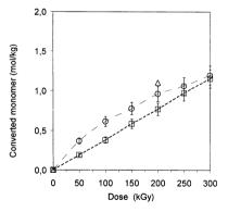
Figure 1. Progress of fractional conversion of AU as a function of EB-irradiation dose, in a SAU20 blend ( $\square$ ) and in the two crystalline forms of AU (O, monoclinic;  $\Delta$ : tetragonal).
